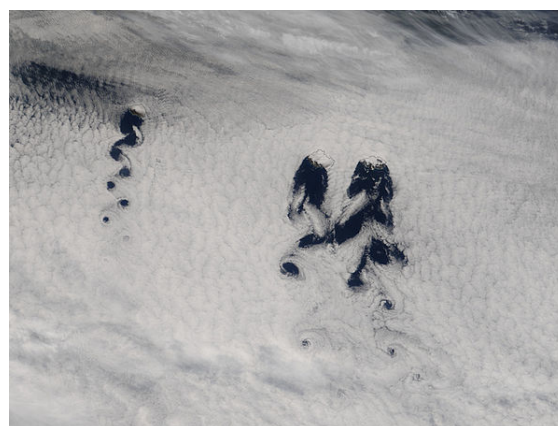
Crozet Islands causing a Von Karman Vortex street to form under low clouds.
